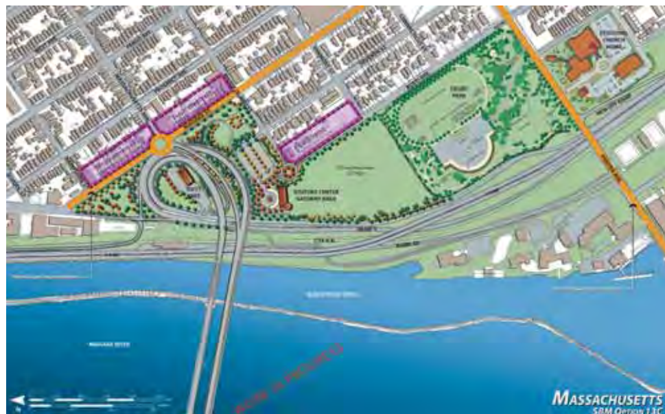
Draft North Alignment: A draft proposal (August 2005) for the Shared Border Management Alternative moves the bridge landing to the north of the initial City of Buffalo investigation. (Source: Fort Erie and Buffalo Public Bridge Authority)
