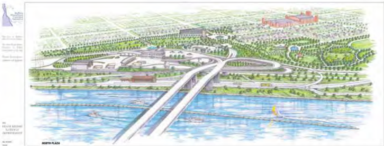
The North Plaza Alternative without shared border management requires the largest land area to accommodate border security and customs as seen in the plan (top) and sketch (bottom).
