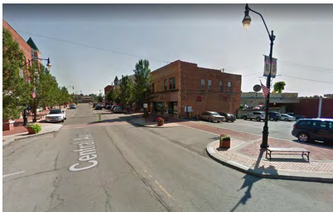
Streetscape improvements on Central Avenue include benches, landscaping, curb bump-outs, crosswalks, and prominent sidewalks to improve walkability
