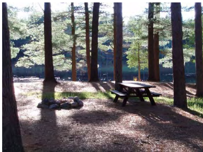
County features a hardened natural surface that meets or exceeds width requirements, a universal picnic table with extended tabletop, a fire ring with raised base and thin walls, a tent pad, and connection to an accessible path (not shown).
