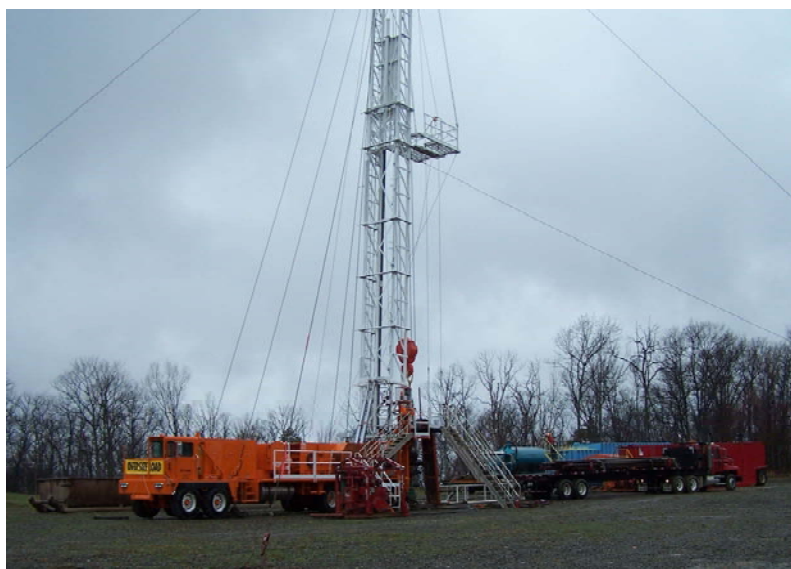
This service rig is an example of the heavy equipment that is needed to drill and work over a natural gas well.
